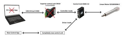
Figure: Expected state after reusing all suitable parts of current setup
