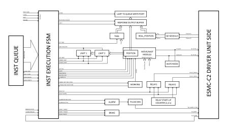
Figure: Block Diagram of Execution Module
